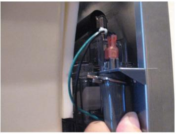
4. Locate drain hose, lower to drain water.
